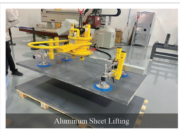
Mechanical Vacuum Lifter (4 Suckers) FS-WDL800-4S (800KG)
