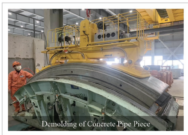
AC-Vacuum Lifter (3 Suckers) FS-M5000-3S (5000KG)
