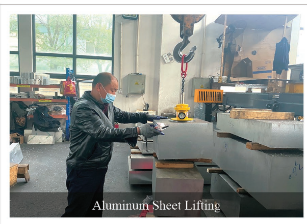
Mechanical Vacuum Lifter (Single Sucker) FS-WDL80-IS (80KG)
