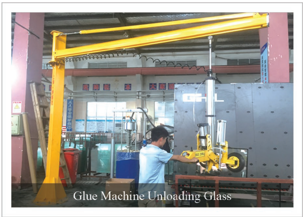
Pneumatic 90°Flip and Rotation (2 Suckers) FS-QFX150-2S (150KG)
