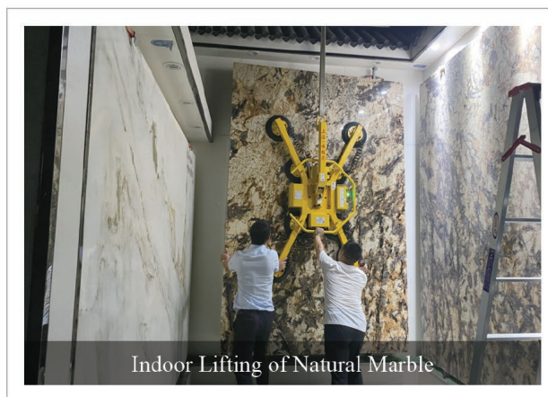
DC-Vacuum Lifter (8 Suckers) FS-MSFX800-8S (800KG)
