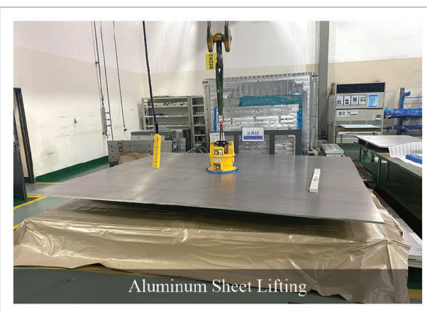
Mechanical Vacuum Lifter (Single Sucker) FS-WDL800-IS (800KG)
