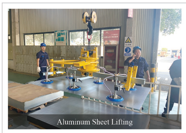
Mechanical Vacuum Lifter (6 Suckers) FS-WDL600-6S (600KG)
