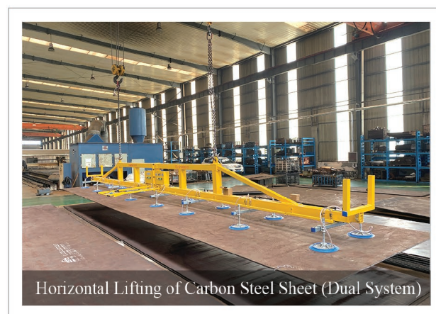
DC-Vacuum Lifter (16 Suckers) FS-BLZ3000-16S (3000KG)
