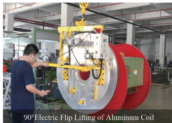
AC-Aluminum Coil Vacuum Lifter(multi-chamber) FS-C1000-3S (1000KG)
