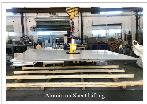
Mechanical Vacuum Lifter (Single Sucker) FS-WDL300-IS (300KG)
