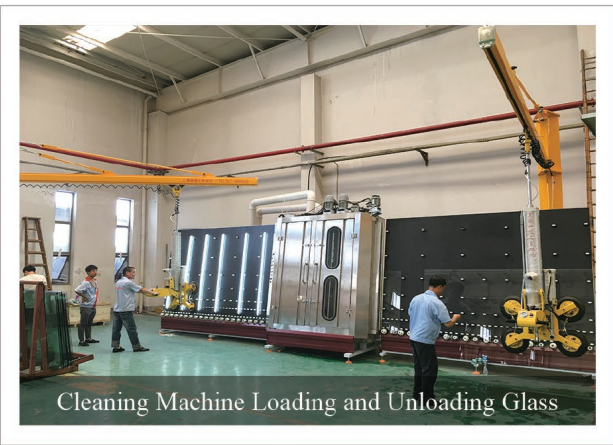
Pneumatic 90°Flip and Rotation (4 Suckers) FS-QFX250-4S (250KG)
