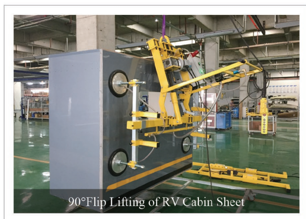
AC-Vacuum Lifter (4 Suckers) FS-WDF400-4S (400KG)
