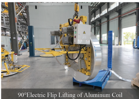
AC-Aluminum Coil Vacuum Lifter(multi-chamber) FS-C1300-3S (1300KG)
