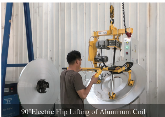
AC-Aluminum Coil Vacuum Lifter(single chamber) FS-C250-1S (250KG)
