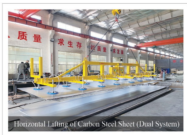
DC-Vacuum Lifter (16 Suckers) FS-BLZ3000-16S (3000KG)
