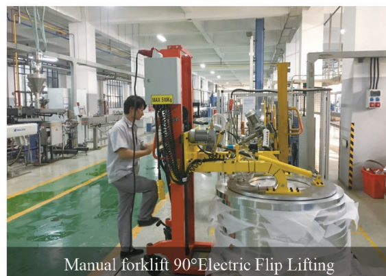
Mobile Aluminum Coil Vacuum Lifter FS-C5000-1S (500KG)
